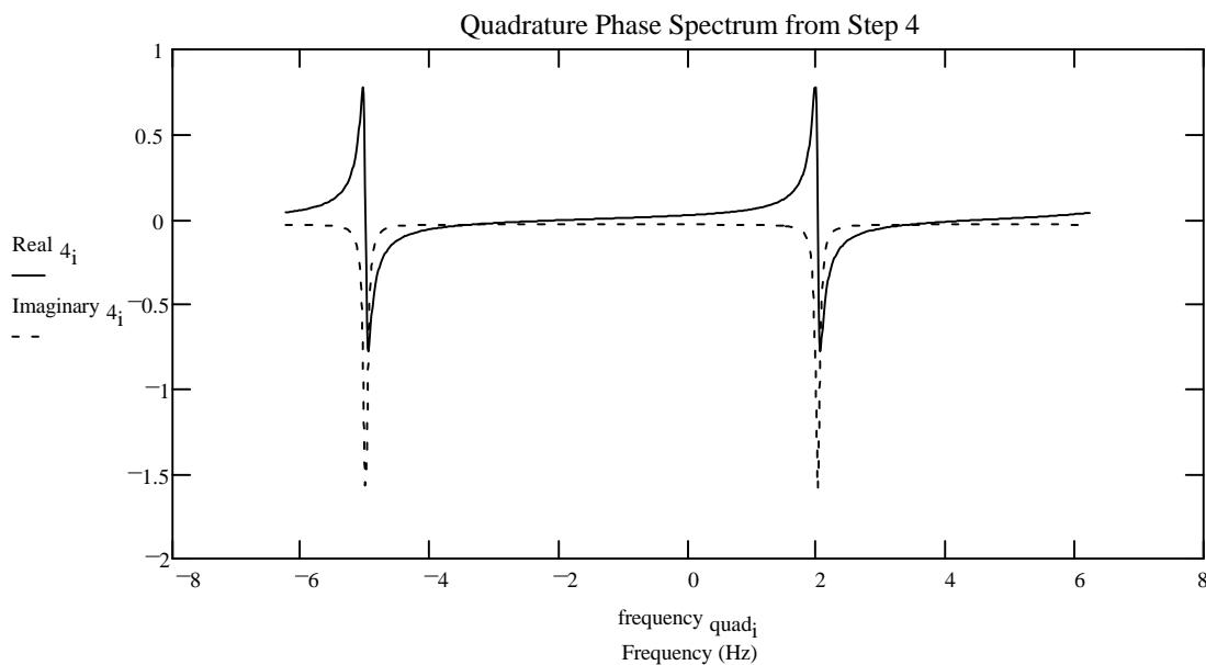
**Phase Cycling Effect.** Finally the spectra collected from each step of the phase cycle are combined to produce the quadrature phase cycled spectrum. Notice that the signals add, but the artifacts have a different phase relationship so they cancel.
