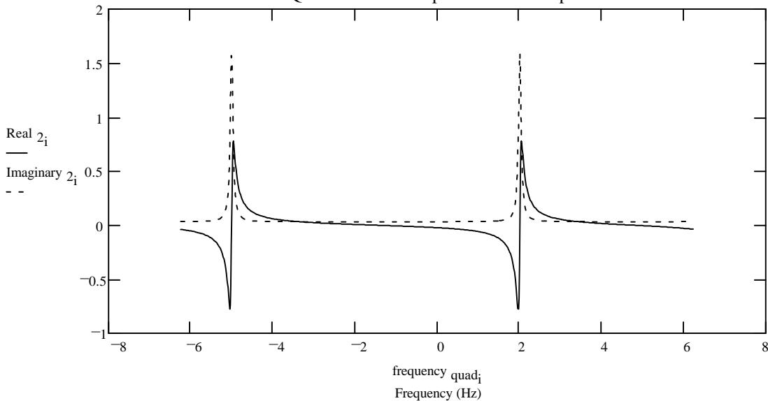
**Third Step 180°.** In the third step of the phase cycle the transmitter phase is at 180 degrees ( $\pi$  rad) relative to the first step.
